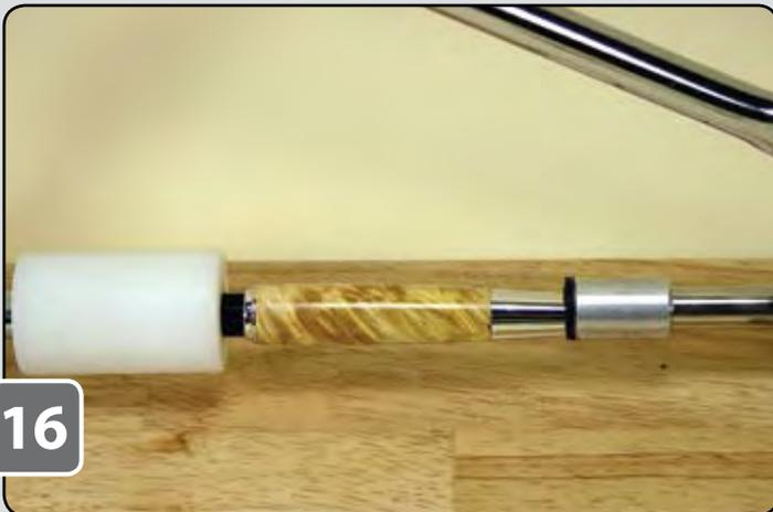
Using a pen press, press the front end coupler and the end cap into the lower portion of the barrel as per the instructions for the pen kit and continue assembling the pen to completion.
