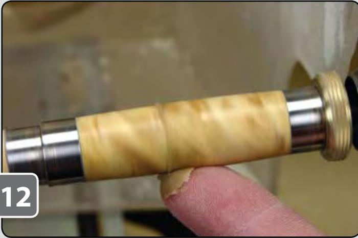
Apply a small amount of EEE Cream on your finger; then apply it to the workpiece with the lathe running at approximately 500 to 700 rpm.
