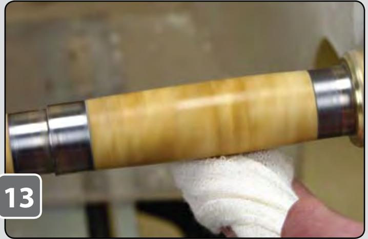
Turn up the speed of the lathe and apply pressure with a cheesecloth to build up some friction, thus sealing the EEE Cream into the pen blank.
