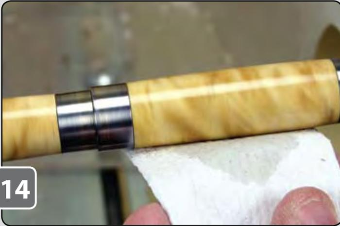
Apply woodturner's finish to a paper towel and, with the lathe running, slowly apply the finish to the entire pen. Then, turn up the speed of the lathe and apply pressure to once again cause some friction to seal the polish into the pen.
