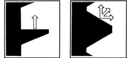
Buttress thread produces pure tensile load
